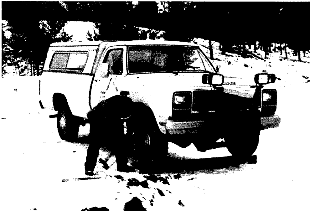
Figure 7. Generating shear waves for the site characterization measurements. The cable leading from the sledgehammer allows the impact time to be recorded.
