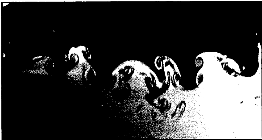
Figure 2.5. Laser-induced fluorescence (Y, Z) cross-section through the braid region of an incompressible planar mixing layer. The entire channel span of 11 cm is shown (from Bernal and Roshko [1986]).
