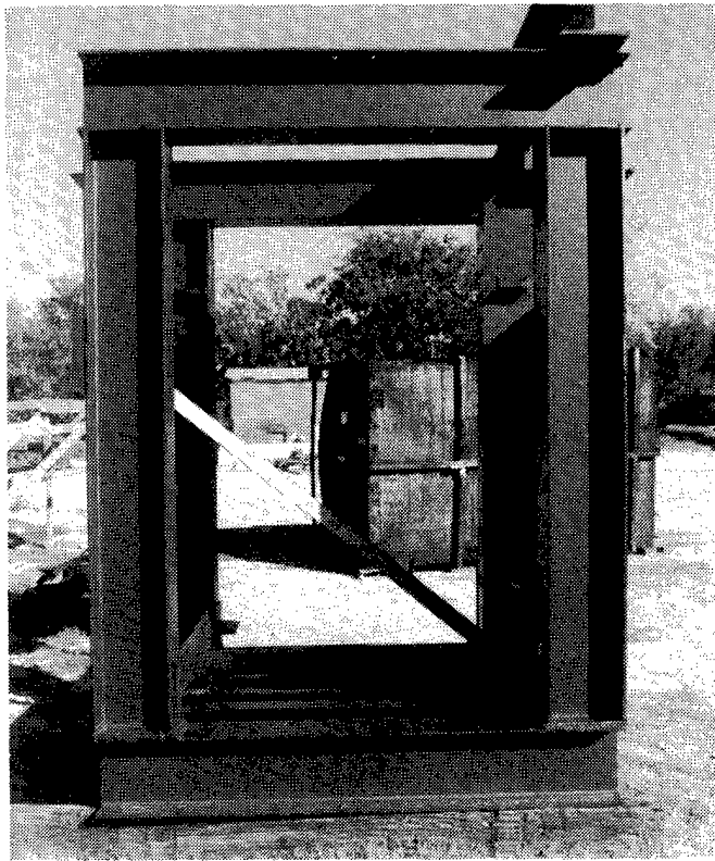
Figure 19. Photograph of the Ballistic Pendulum Fixture, Showing the Rails Used to Interpret Pendulum Swing.
