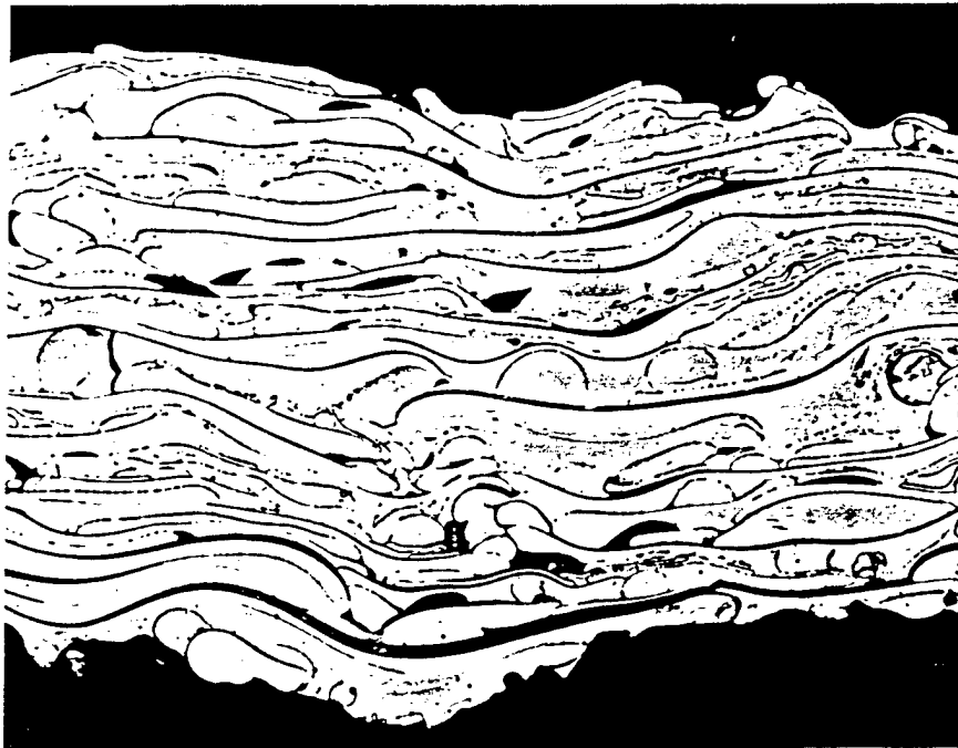
Figure 4.2-5. (Specimen A3, 500X) Cross section of Versalloy 50 coating in as sprayed condition.
