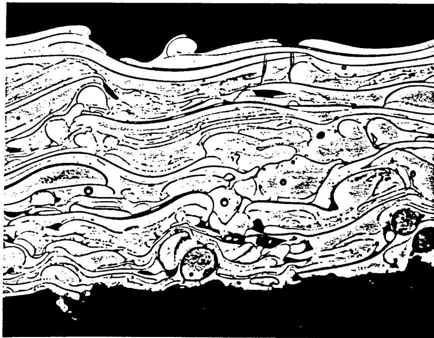
Figure 4.2-6. (Specimen A3, 500X) Cross section of Versalloy 50 coating in as sprayed condition.
