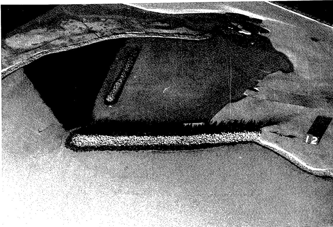
Photo 7. Placement of tracer material for existing conditions prior to model testing
