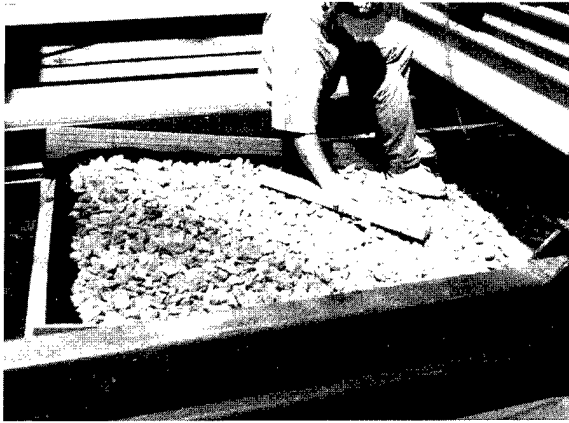
Figure 14. Leveling rocks of model riprap in final preparation prior to each test.
