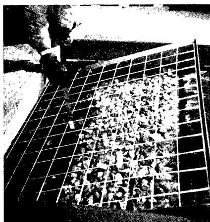
Figure 13. Measurement of the distance of the riprap surface from the strings at each grid point.
