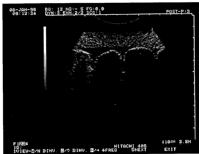
Figure 4. B-Scan Image of Blood Pool Phantom (3.5 MHz)
