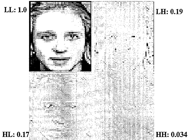
Figure 6.3: Different components of a wavelet transform, capturing sharp variations of the image intensity in different directions, have different discriminatory potentials. The numbers represent the relative discriminatory power.
