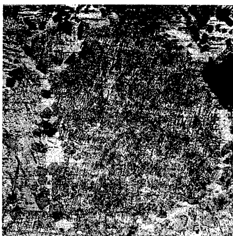
Fig. 33--Same Sample as Shown in Fig. 31, Annealed at 1625°C for 60 Minutes, Air-Etched, X 250.
