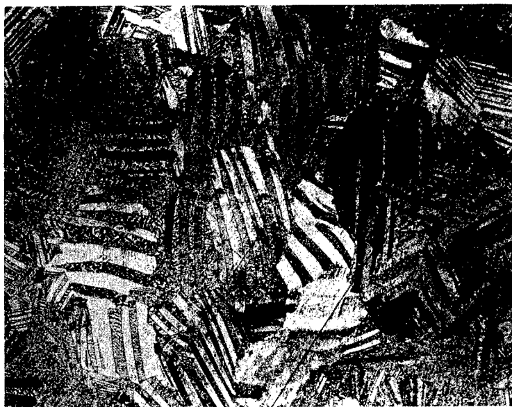
Fig. 12--Typical Structure of \text{ThC}_2 , Air-Etched, X 90
