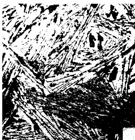
Fig. 34--ThC 2 -C Eutectic Containing Approximately 12.6% Carbon, Furnace-Cooled, Unetched, X 100.
