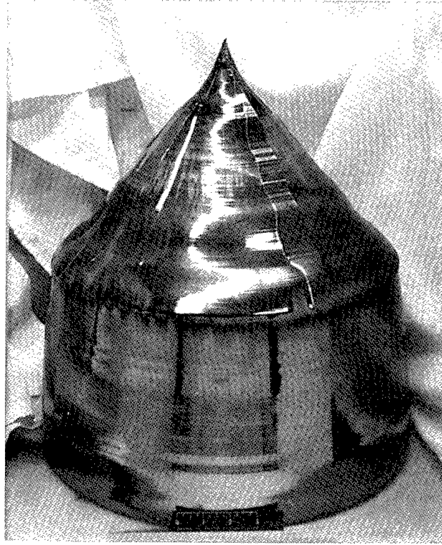
Figure 3. Single-Crystal Silicon Boule Fabricated for the Monolithic Inner Cone
