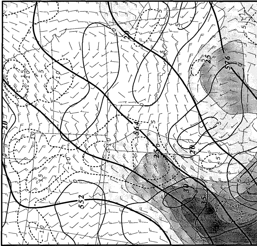
Figure 3.31. 60 km full physics 500 mb MASS model output valid at 1500 UTC 8 March 1992. Parameters depicted: heights (solid - 6 dm interval), total wind isotachs above 20 \text{ ms}^{-1} (shading at a 5 \text{ ms}^{-1} interval), ageostrophic wind barbs (flag - 25 \text{ ms}^{-1} , full staff - 5 \text{ ms}^{-1} , half staff - 2.5 \text{ ms}^{-1} ), and kinematic omega where ascent is depicted by dashed line and descent is depicted by thin solid lines ( \mu\text{bar s}^{-1} ).
