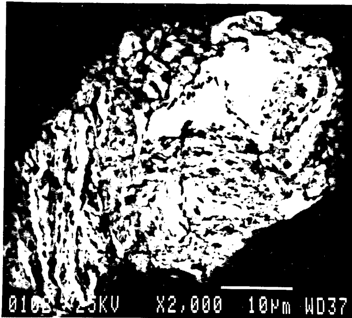
Figure 6 SEM micrograph of Nb-Si mixture milled for 1 hr.
