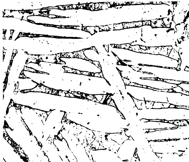
Fig. 11—Copper-zirconium alloy (bomb-reduced). 0.76% copper, 150X Annealed and quenched at 920°C.
