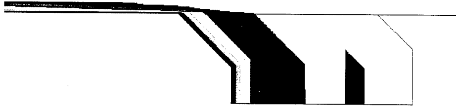
Figure 4.7: Current distribution in the segmented copper fibre armature consisting of 3 segments at t = 0.25415 s ( v = 729.6 m/s).
