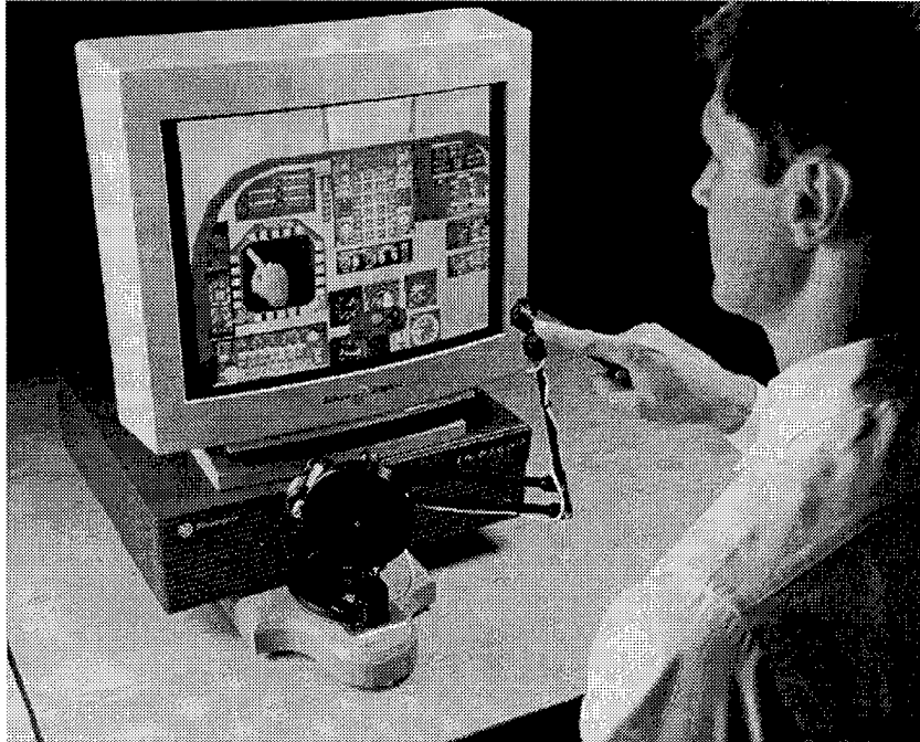
Figure 5: The Virtual Maintenance Trainer allows the user to push buttons, throw toggle switches, turn dials, observe lights, and listen to audible tones, and manipulate linkages during the evaluation and adjustment of aircraft systems.
