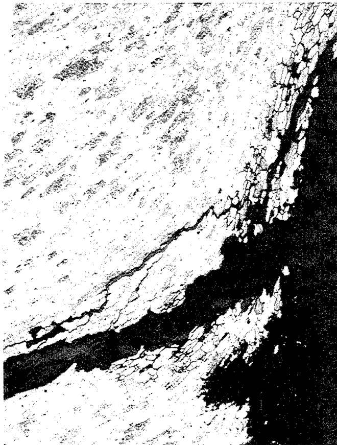
Figure 45. Etched microstructure of the same area in Figure 44, showing the grain flow formed by the head-forming operation. Magnification: 100×. Keller's etchant.
