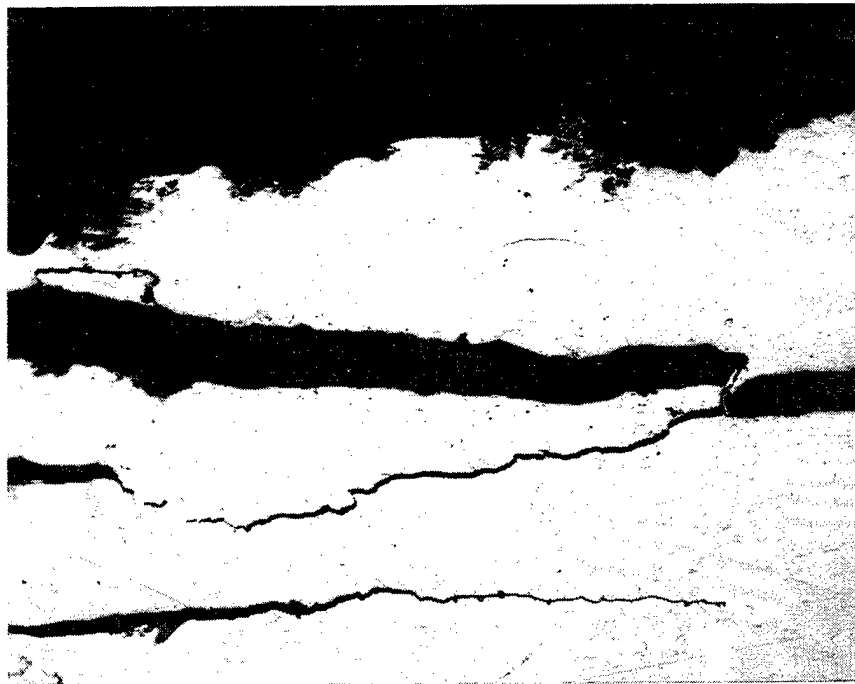
Figure 13. As-polished microstructure at the bottom of the corroded hole in Figure 11. Exfoliation was the primary mode of corrosion on the corroded surface of the angle section of the AVLB top chord. Magnification: 75 \times .
