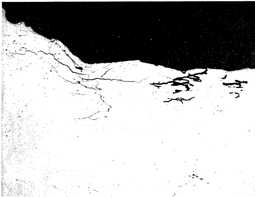
Figure 9. As-polished microstructure of the aluminum rivet in Figure 8. Intergranular corrosion and cracks are present in the small corroded area in head-to-shank fillet, indicative of stress corrosion cracking. Magnification: 170x.
