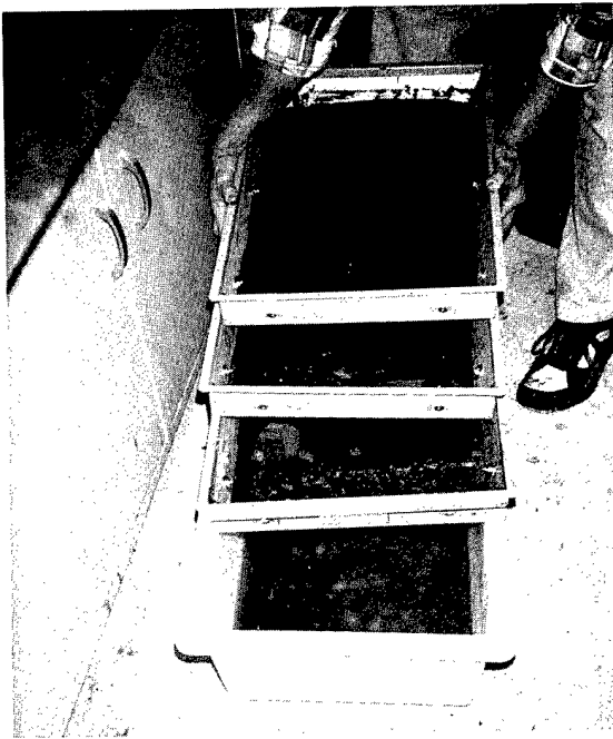
Figure 6. Nest of sieves (no. 30, 50 and 100) used to concentrate alum sludge to 6% and 12% total solids.
