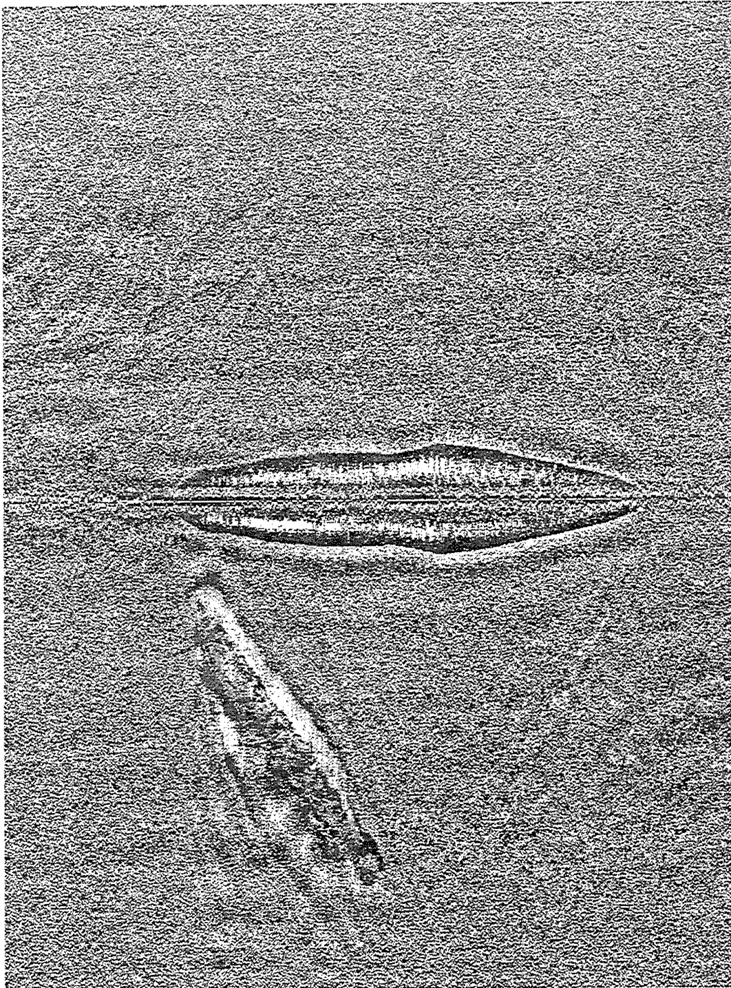
Figure 5. The "fine details" image, corresponding to the subtraction of the across-track filtered image (Figure 4) from the original sonogram (Figure 1).
