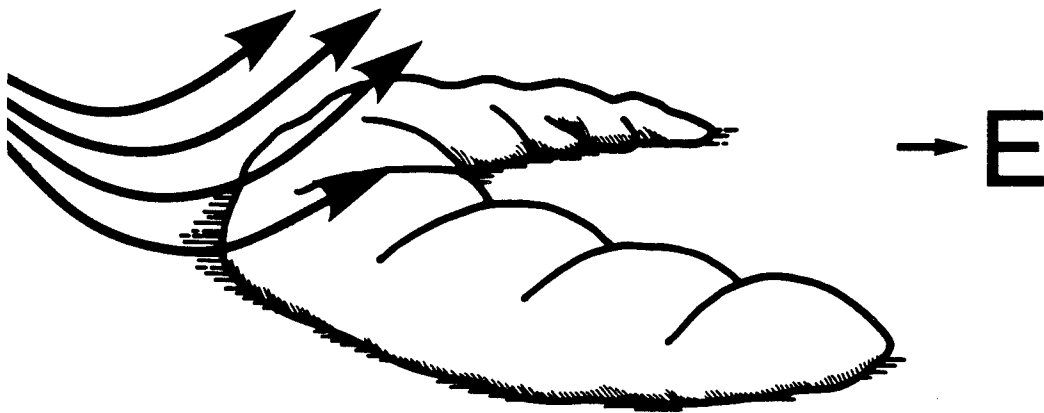
Figure 3.3-15. Windbreak effect of land contouring (after Kerr, no date).
