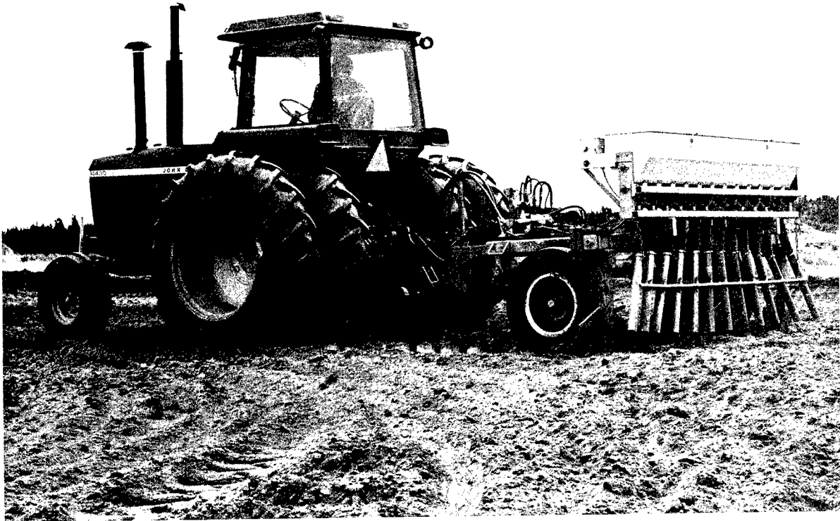
Figure 3.3-3. Tractor-drawn modified Hodder Gouger (Photo courtesy of U.S. Forest Service Equipment Development Center, Missoula, MT).
