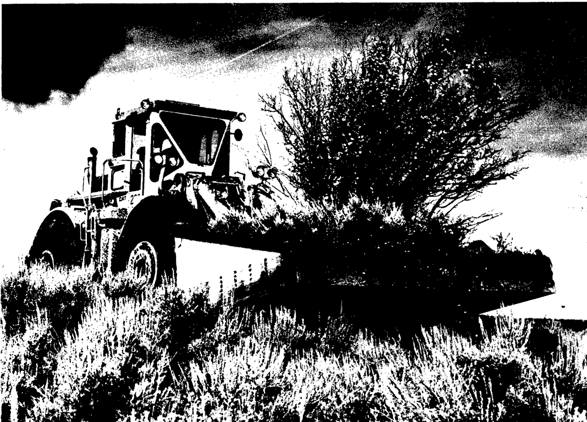
Figure 3.3-2. Front end loader and transplant bucket (photo courtesy of U.S. Forest Service).
