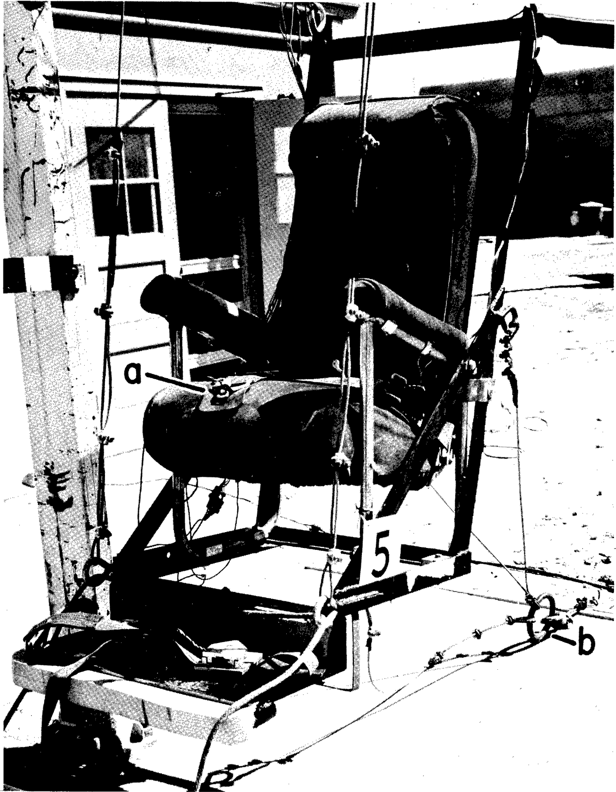
Swing Seat with a. Three-Inch-Wide Lap Belt b. Snub Cable Decelerator
