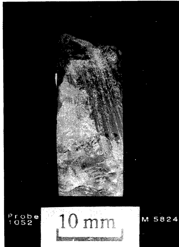
Fig. 6.1 Corner crack, # 1052, 114 m/s
