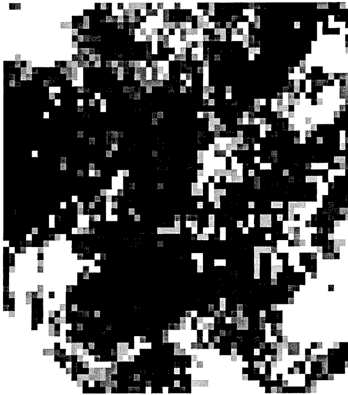
Figure 10: The RTNEPH data after interpolation with the same data used in Figure 8 and Figure 9. The data is now displayed in the properly arranged 64 x 64 grid points to match the horizontal resolution of the RWM. RTNEPH data now has the same resolution as the RWM as described in the text.
