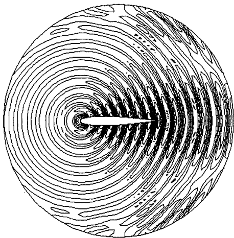
Figure 7. Scattered electric field intensity, E^z , about the NACA0012 airfoil.
