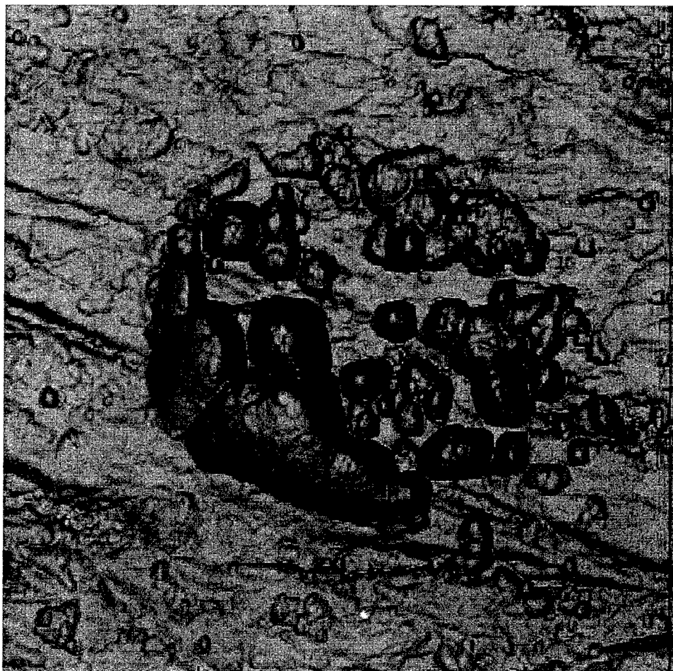
FIGURE 4 Scanning Force Microscopy image of the \text{CaF}_2 surface irradiated with 0.9 keV electrons, 3.3 \times 3.3 \mu\text{m}^2 , irradiated with 1.5 \mu\text{A} for 200 sec.
