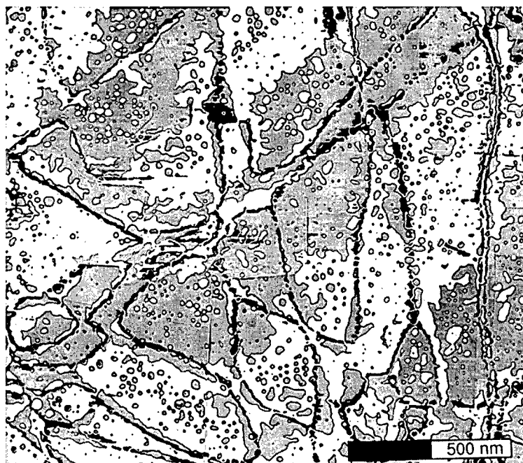
Fig. 6. Modified representation of the STM image shown in Fig. 4 with enhanced contrast between regular surface areas (alternating white/grey), and surface areas displaced by the strain fields of misfit dislocations (black). The grey scale in the image is adjusted such that surface areas with a height within intervals of (n \times d_{ML}) \pm \Delta appear alternating white/grey ( n : integer number and \Delta = d_{ML}/10 ), whereas surface areas with other z -values appear black.
