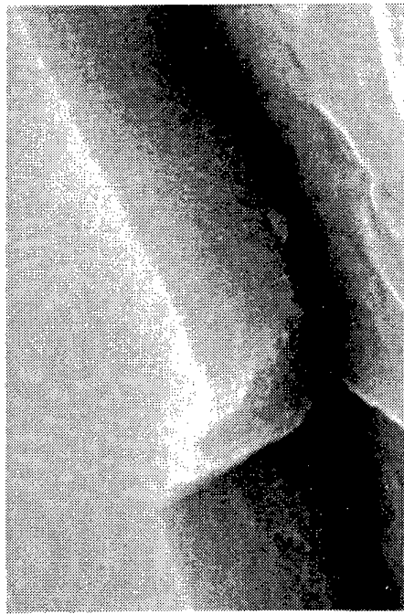
Figure 3. Photographs of cross sections of sputter-deposited MoS 2 films, showing the effect of film doping on structure. The cross sections are produced by fracturing the films using a Rockwell indenter. Shown are (a) pure rf-sputtered MoS 2 , (b) DC-sputtered MoS 2 cosputtered with Ni, and (c) rf-magnetron-sputtered multilayers consisting of alternating layers of MoS 2 and Ni.
