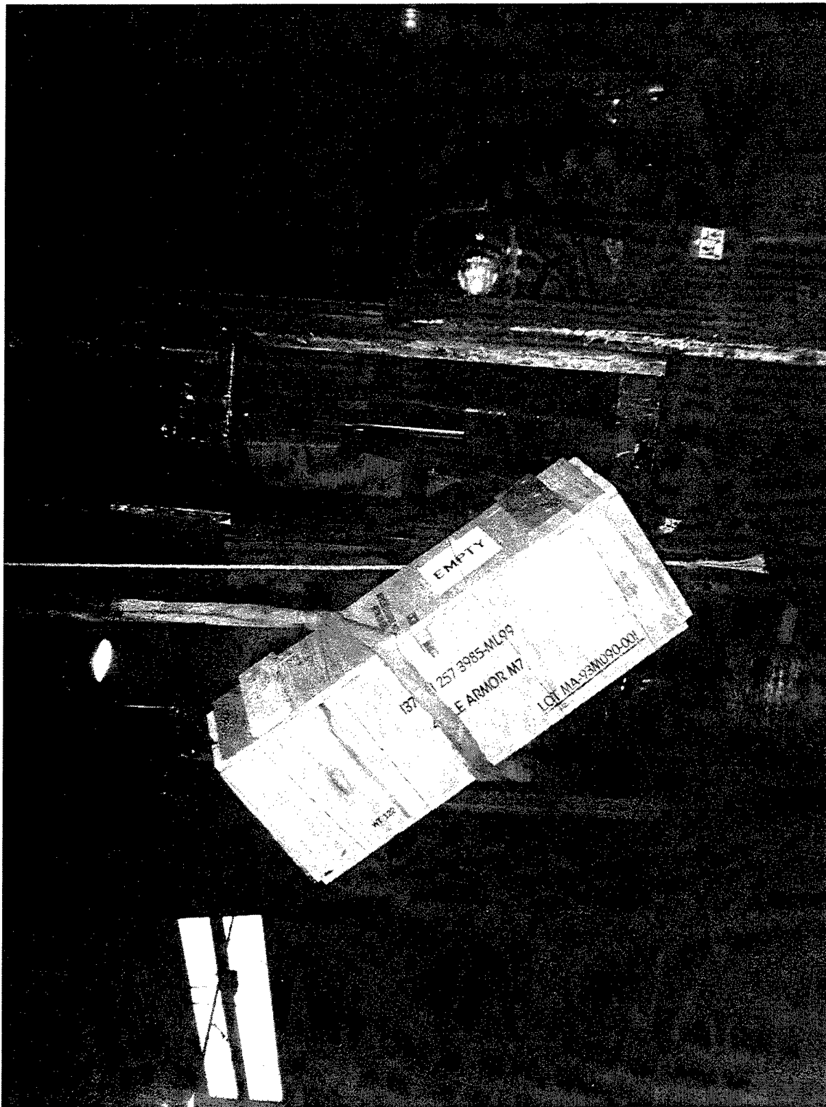
U.S. ARMY DEFENSE AMMUNITION CENTER AND SCHOOL - SAVANNA, IL AO317-SPN-96-089-1122. This photograph shows the armor tile box with four bundling wires raised to 3.9 feet for the 45-degree angle drop required for UN POP certification.
