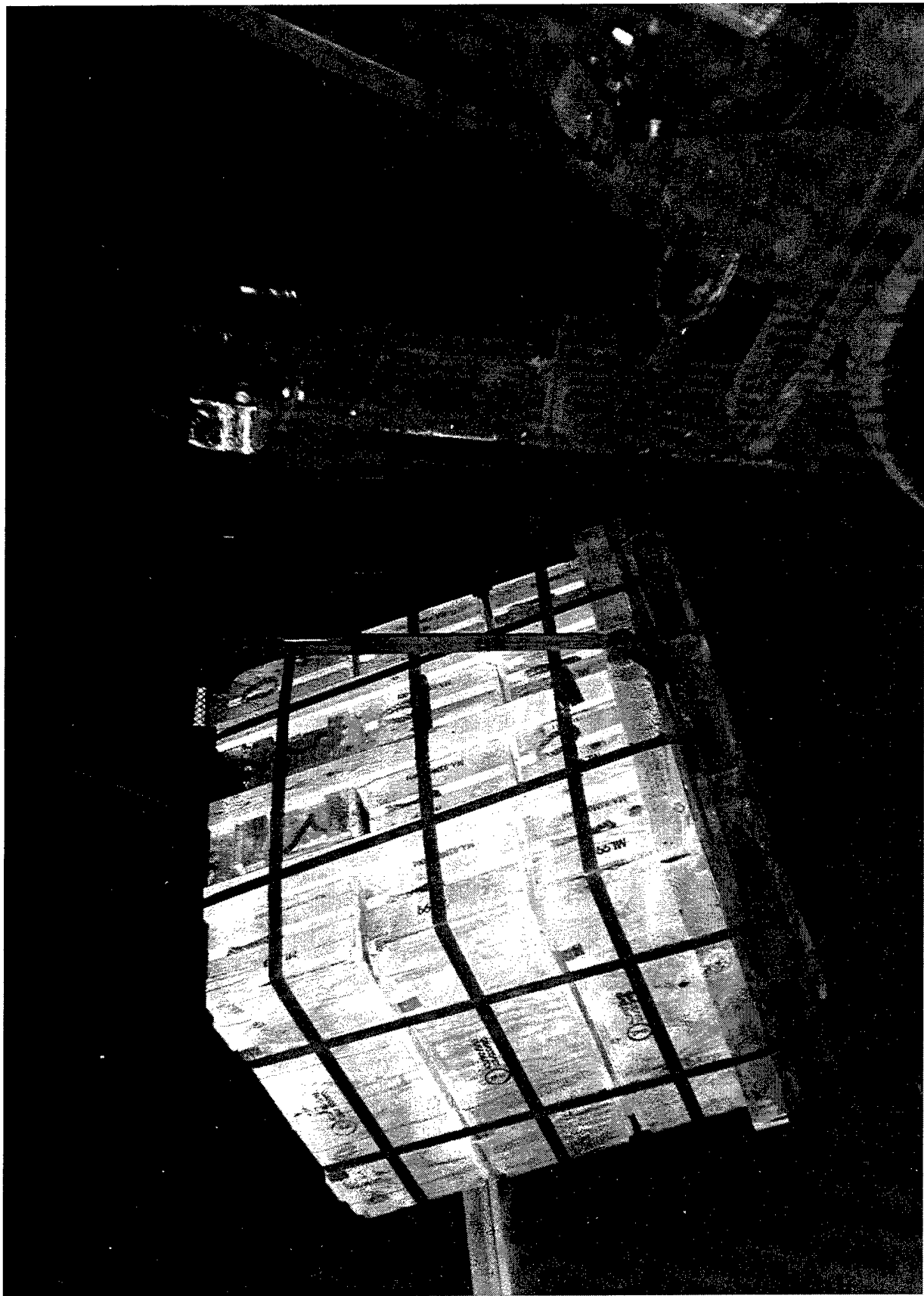
U.S. ARMY DEFENSE AMMUNITION CENTER AND SCHOOL - SAVANNA, IL AO317-SPN-96-089-1156. This photograph shows the armor tile pallet (palletization method no. 1) raised in preparation for the edgewise rotational drop test.
