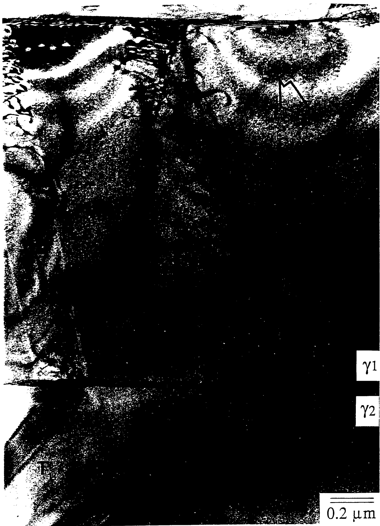
Shielding of a crack tip in a two-phase ( \alpha_2+\gamma ) titanium aluminide alloy by deformation twins and (1/2) \langle 110 \rangle dislocations (CM 3334).
