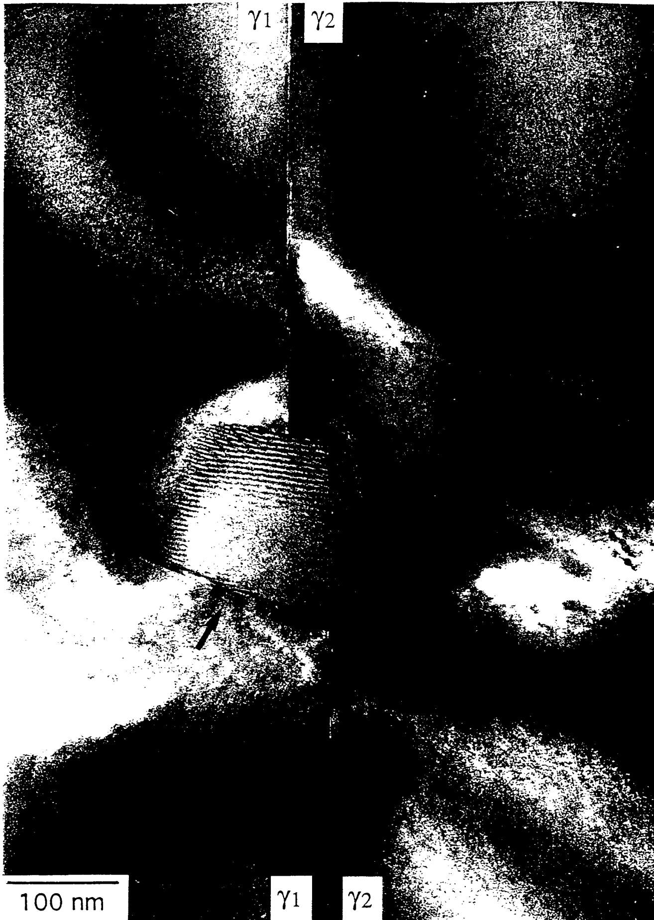
Recrystallized \gamma grain within a lamellar colony of a Ti-48at.%Al-2at.%Cr alloy. Creep deformation: \sigma = 140 MPa, T = 700 °C, t = 6000 h, \epsilon = 0.69\% . (CM 4216)
