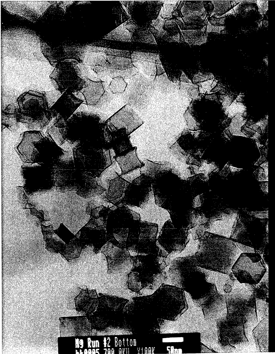
Figure 11. TEM micrograph of a second sample of magnesium powder obtained from the bottom of the collecting rod. For calibration, the white bar at the bottom is 50 nanometers.
