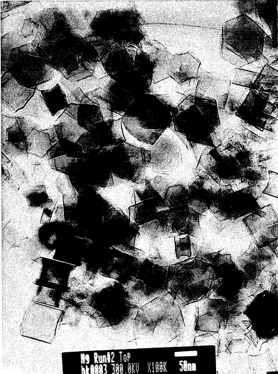
Figure 13. TEM micrograph of a sample of magnesium powder obtained from the top region of the collecting rod. For calibration, the white bar at the bottom is 50 nanometers.
