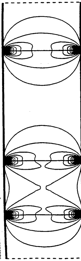
Figure 2. Distribution in terms of isostress contours of the stress component normal to the grain boundaries in the conductor of Fig. 1.
