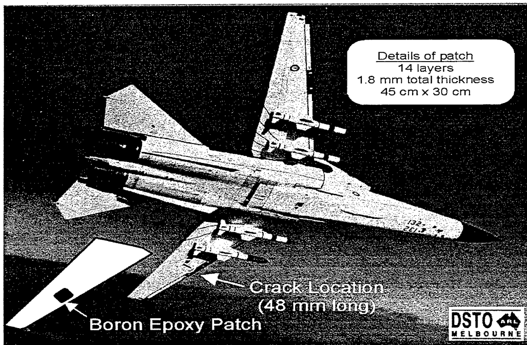
Figure 2. Boron Epoxy Patch Repair to RAAF F-111
