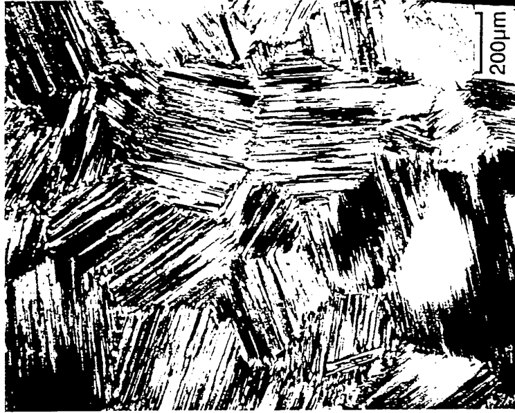
Cooling Condition Effect on RFL of Alloy K5
