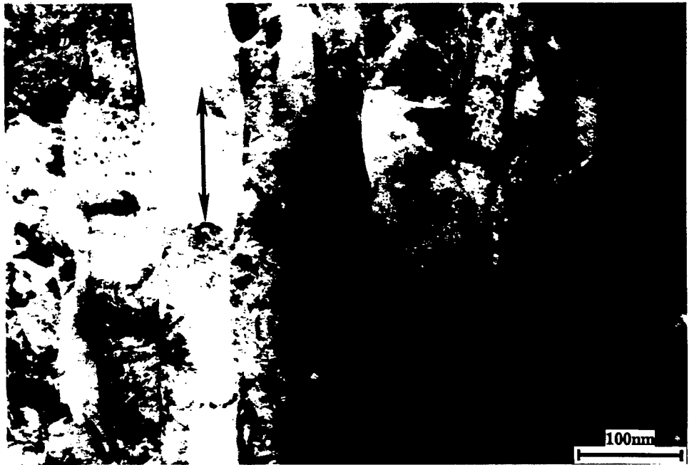
Figure 5. Shear band microstructure. (a) Elongated grains extending in the shear direction (arrow). (b) Enlarged view of elongated grains within the shear band showing finely dispersed second-phase particles, possibly carbides.
