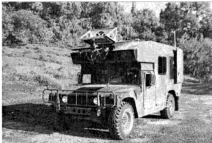
Figure 1.3 The Navlab 2, a converted army HMMWV
