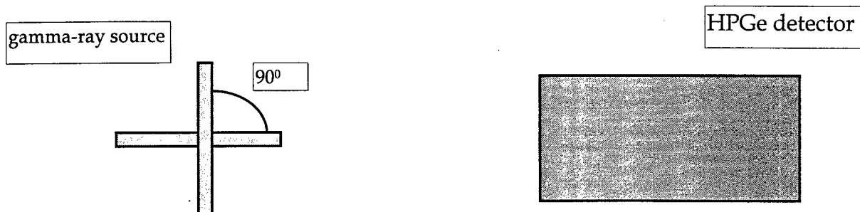
Fig. 1. Schematic representation of the experimental set-up, which rotates the gamma-ray source 90^\circ to the right every time, when the exposure is over.
