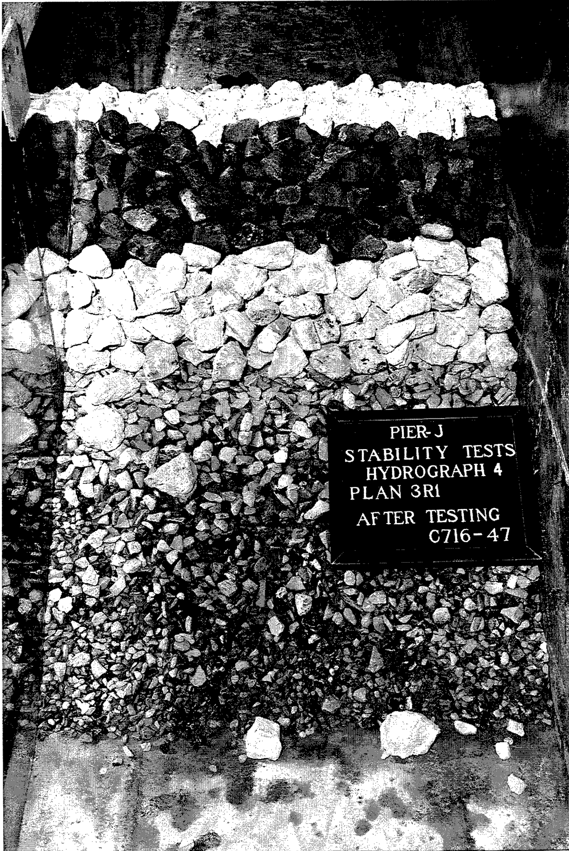
Photo 39. Harbor-side view of Plan 3R1 at the conclusion of testing
