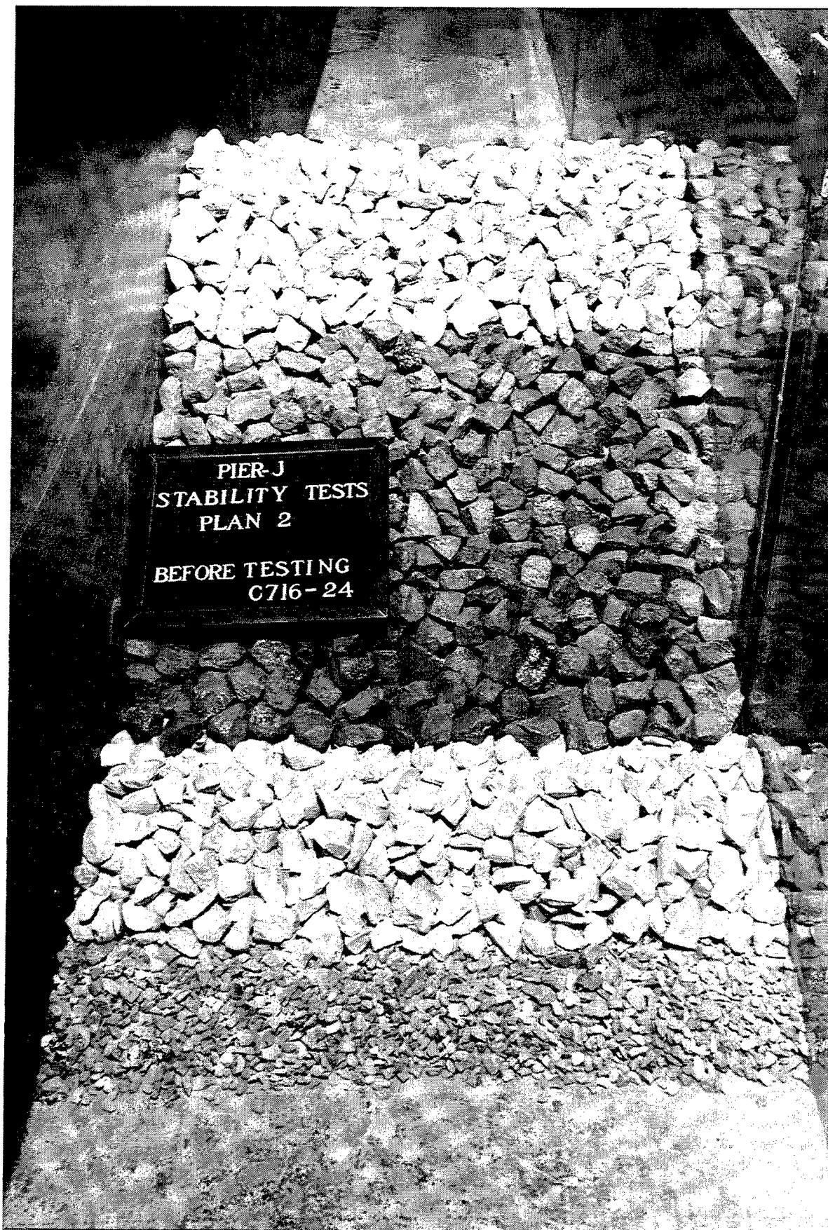
Photo 18. Sea-side view of Plan 2 before wave attack
