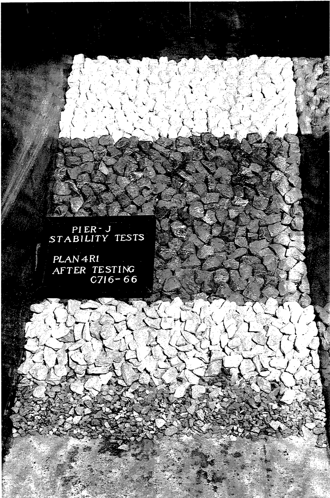
Photo 53. Sea-side view of Plan 4R1 after testing step 14 of Hydrograph 3A
