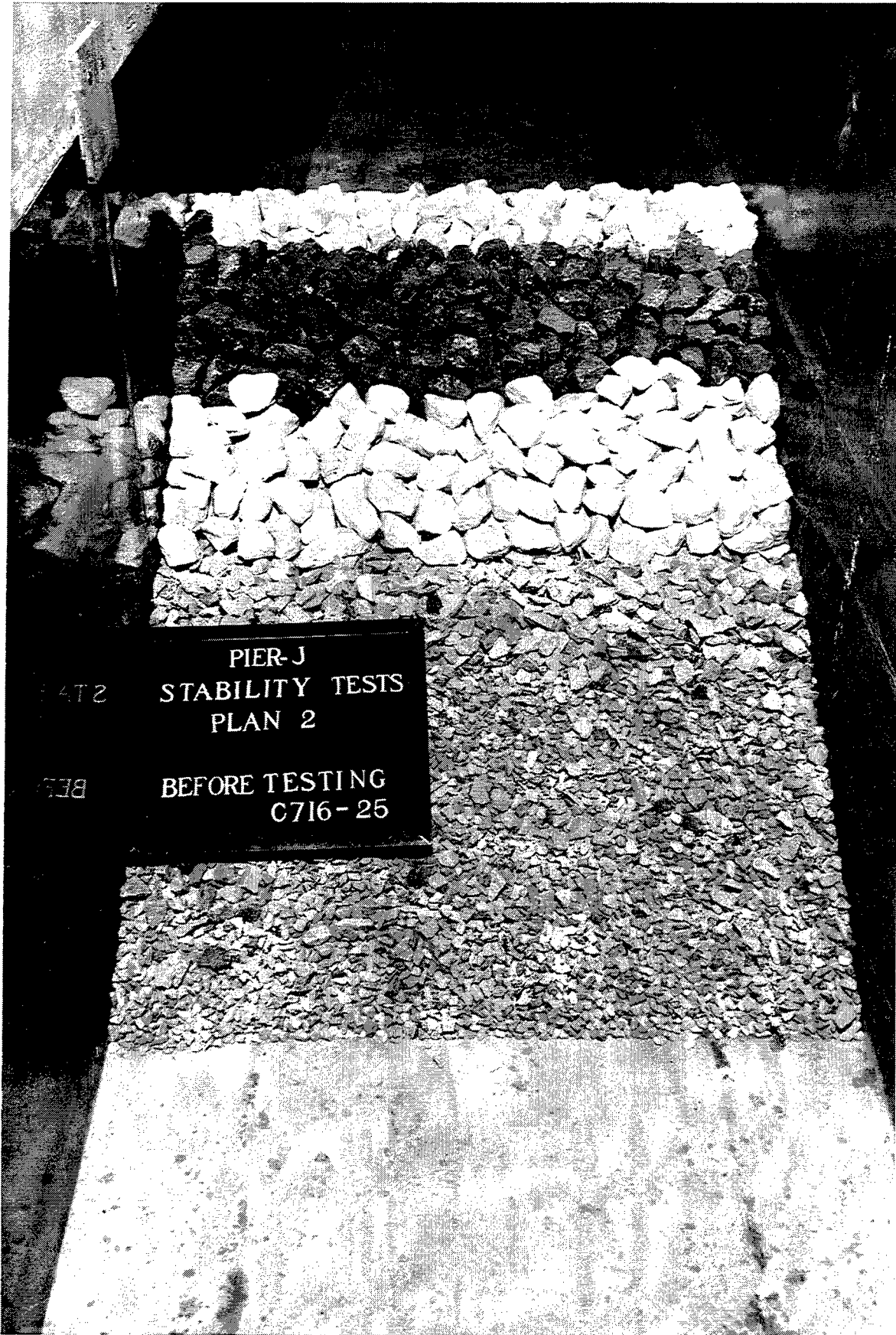
Photo 19. Harbor-side view of Plan 2 before wave attack
