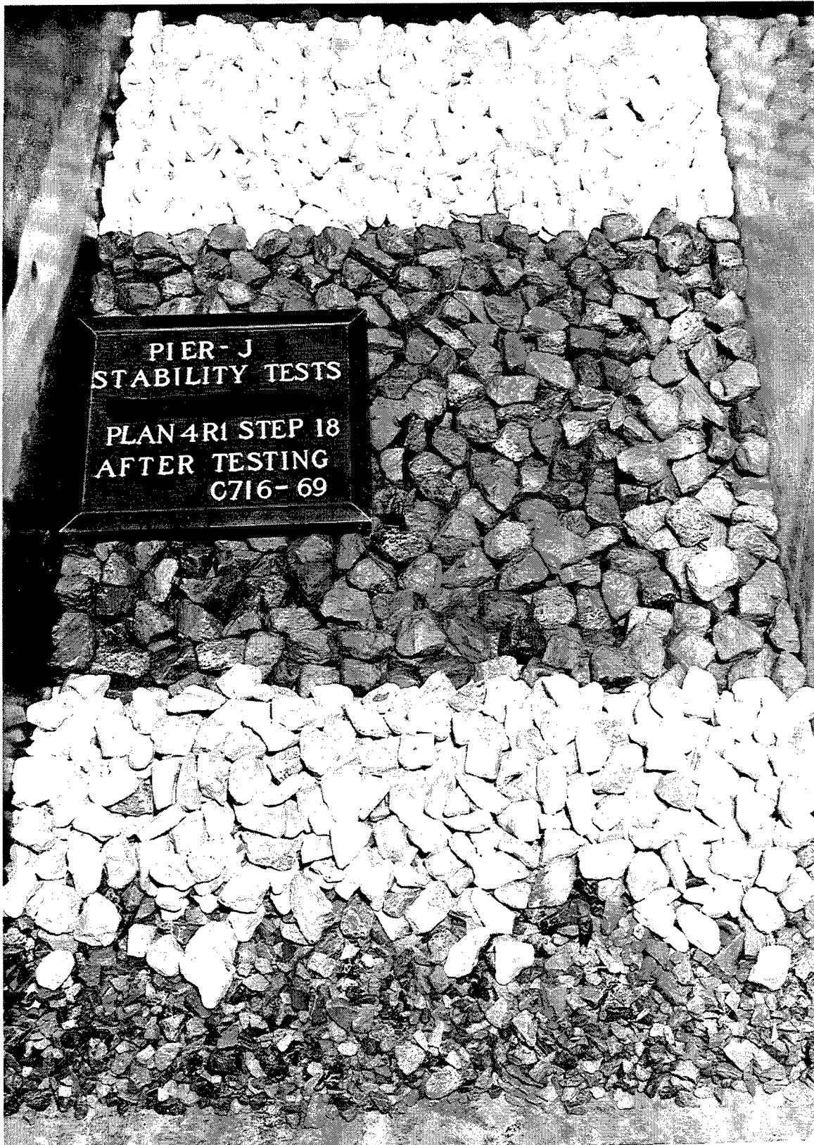
Photo 55. Sea-side view of Plan 4R1 after testing step 18 of Hydrograph 3A
