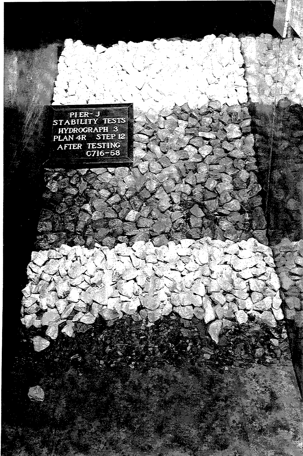
Photo 49. Sea-side view of Plan 4R after testing step 12 of Hydrograph 3
