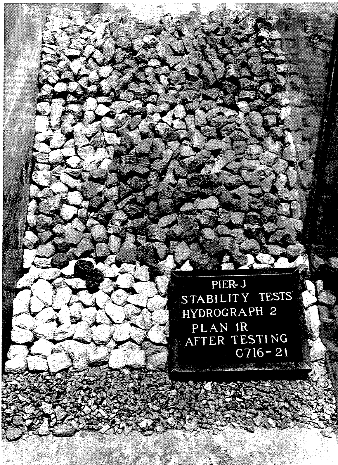
Photo 15. Sea-side view of Plan 1R at the conclusion of testing
