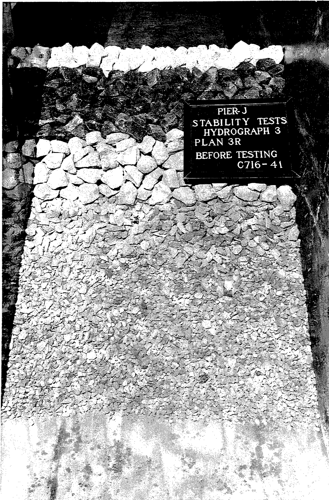
Photo 33. Harbor-side view of Plan 3R before wave attack
