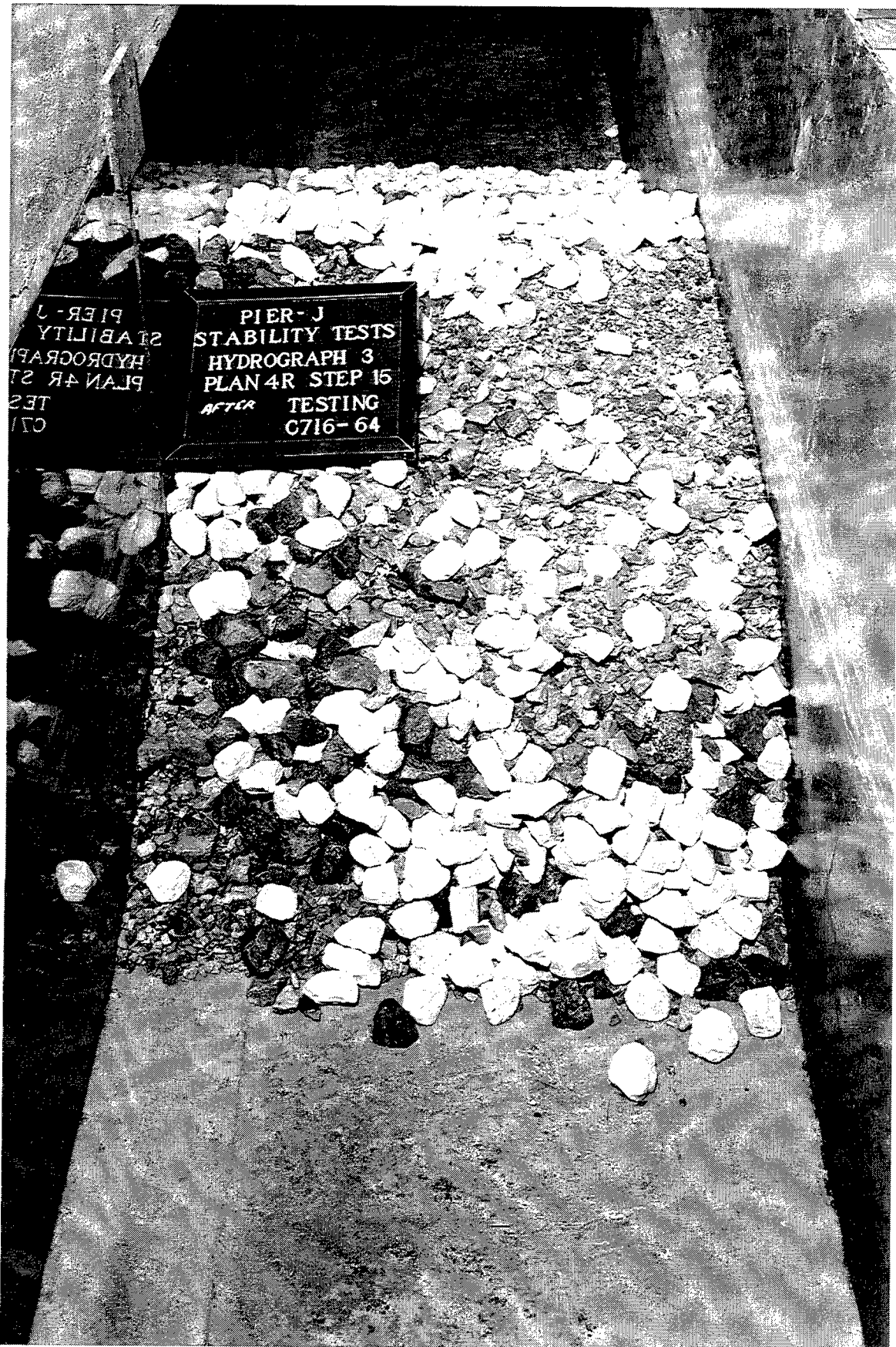
Photo 52. Harbor-side view of Plan 4R after testing step 15 of Hydrograph 3
