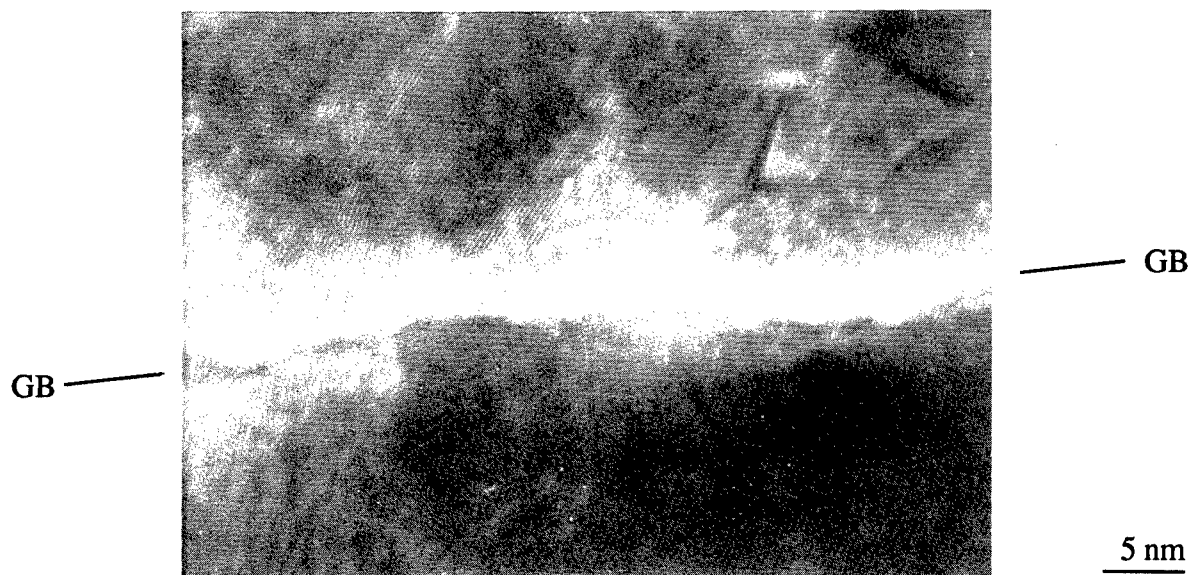
Fig. 3. High resolution TEM lattice image showing a crack propagating through a grain boundary in nanocrystalline gold, d = 8 nm.
