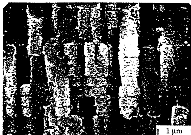
Fig. 2. SEM micrographs of surface and cross-sectional morphologies of a 11.3- \mu\text{m} -thick PZT film.
