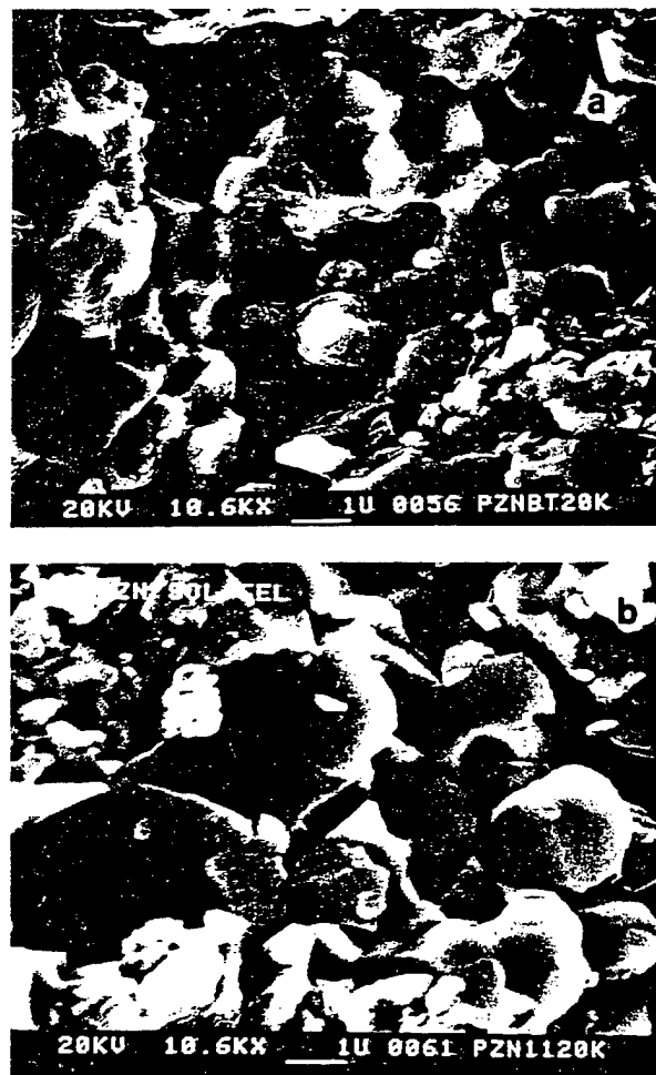
FIGURE 5 Scanning electron micrographs of (a) PZN-BT ceramic and (b) PZN ceramic.
