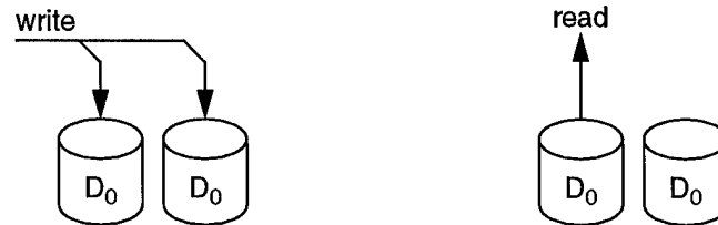
Figure 2-7 Writing and reading data in a mirrored disk array
