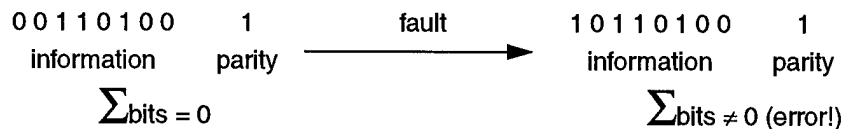
Figure 2-1 Parity codes detect single errors
