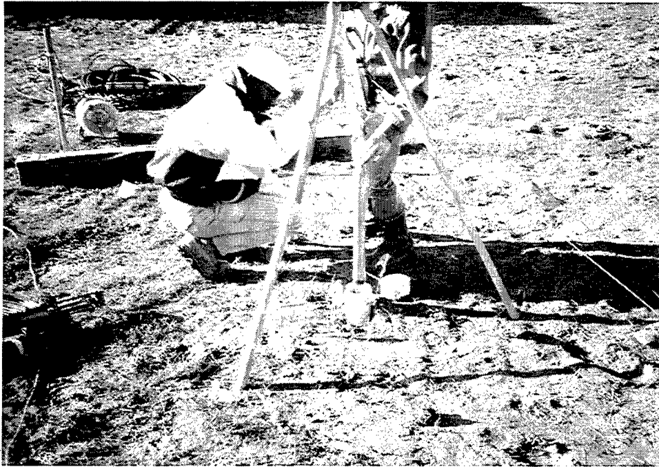
a. Deviation probe being lowered into boring
