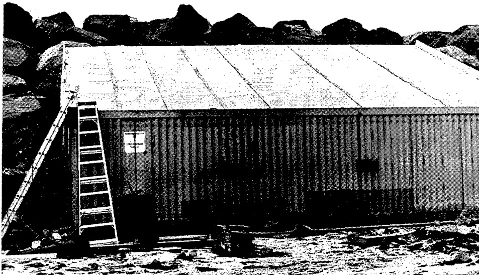
Figure 19. View of collection box used for measurement of wave overtopping
