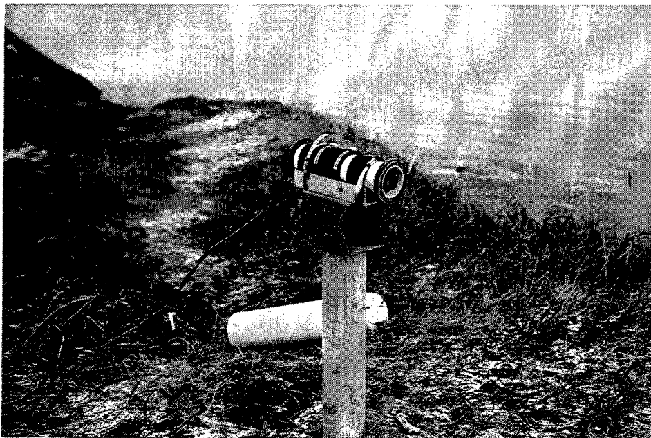
Figure 17. Video camera used to obtain runup data
