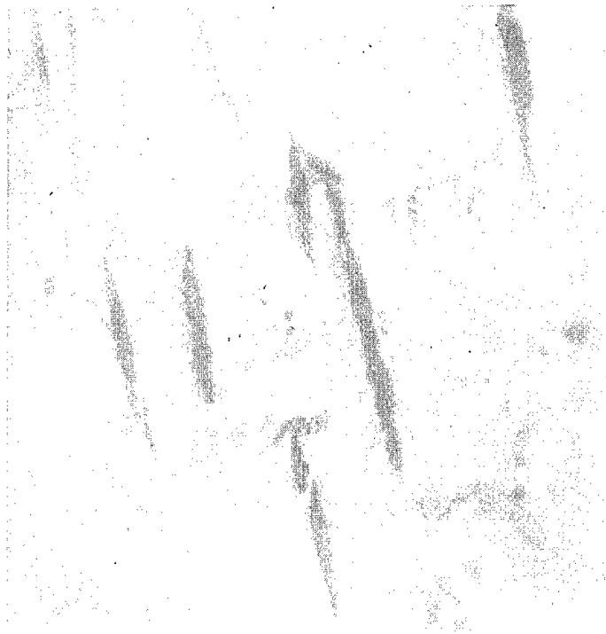
(a) Extracted \gamma'' particles.
