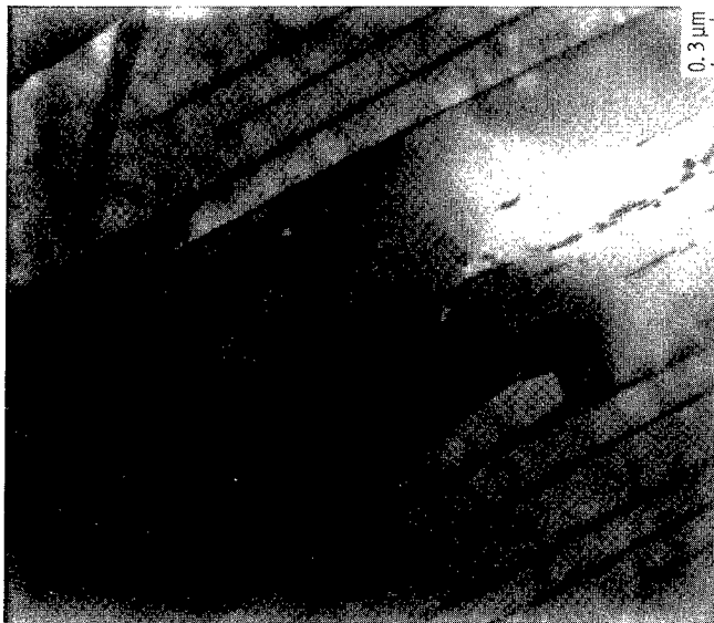
(a) Bright field electron micrograph of fine precipitates observed in \delta regions.
