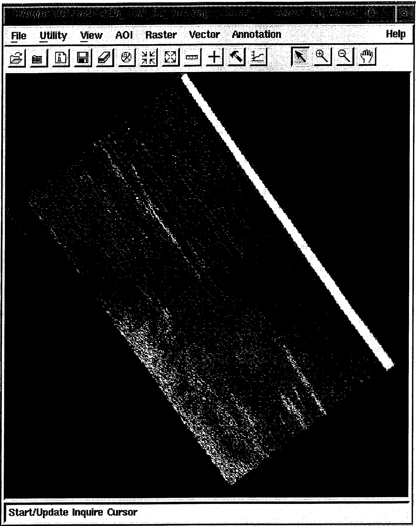
Figure 5c. Geo-rectified, merged Pre- and Post-AGC, AN/SQS-53B imagery for 052° look direction.
