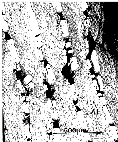
Figure 6. Side view of the fractured tensile specimen of the Al-27vol% NiAl composite (Al=0.250 mm) showing multiple cracks in the aluminide layer. This composite was fracture resistant.
