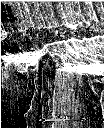
Figure 5. Fracture surface of the Al-40vol% NiAl composite (Al=0.125 mm). Even though this composite displayed little fracture resistance, the Al layers failed in a ductile manner.
