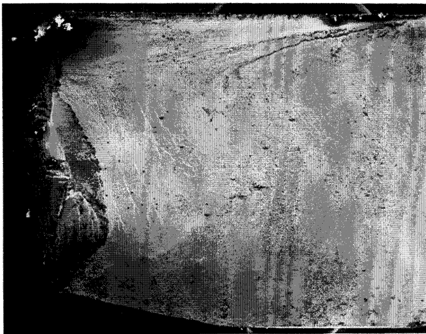
Figure 25. Scanning Electron Micrograph of a Portion of a Secondary Fracture Surface. (This fracture occurred in the damping ring groove region, most likely from a grinding crack. The fracture surface contained an intergranular morphology within the carburized case, followed by a fatigue zone, and finally an overload region toward the center of the piece; magnification 20x.)
