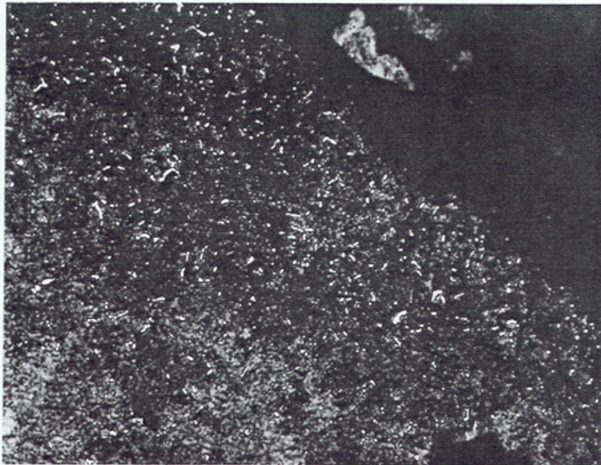
Figure 13. Micrograph of the Gear Tooth Metallographic Sample Showing the Case Microstructure Within Area 3 (Vilella's reagent; magnification 400x).
