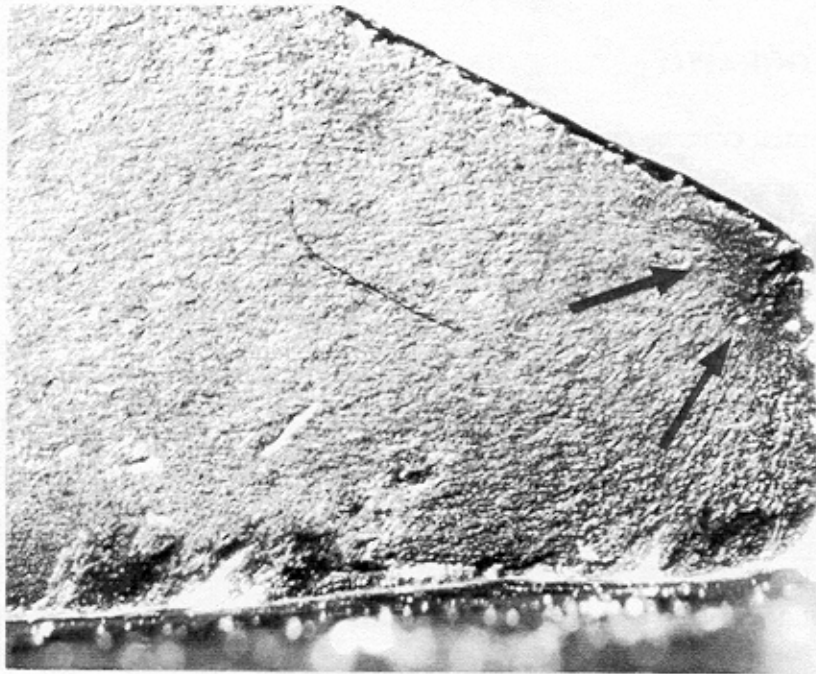
Figure 3. Magnified View of the Processing Defect Located at the Origin. (The grinding crack is denoted by arrows; magnification 40x.)
