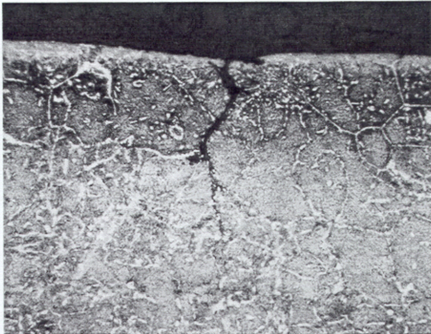
Figure 20. Micrograph of an Intergranular Crack Propagating Along a Carbide Network Noted in Gear P216. (This was not the failed gear being investigated, but this sample provided an example of a grinding crack following the path of a carbide network in X-2M steel; Vilella's reagent; magnification 400x.)
