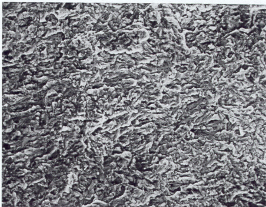
Figure 22. Scanning Electron Micrograph of the Fatigue Morphology, Predominant on the Primary Fracture Surface (magnification 1000x).
