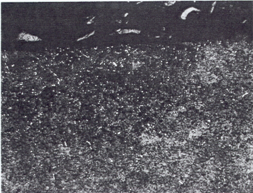
Figure 14. Micrograph of the Gear Tooth Metallographic Sample Showing the Case Microstructure Within Area 4 (Vilella's reagent; magnification 400x).
