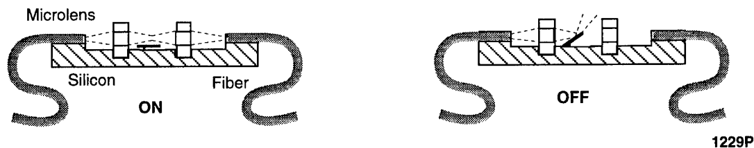
Figure 6. Conceptual drawing of shutter-based in-line fiber-optic crossbar switch system.
