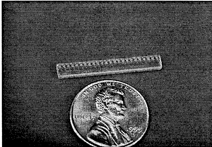
Figure 31. Photograph of 24 element aspheric refractive microlens array.
