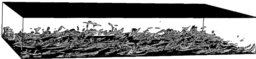
(a) Three-dimensional visualization. For clarity, discriminant is marked only in the lower half of the domain. Flow is from left to right, walls are shaded.
