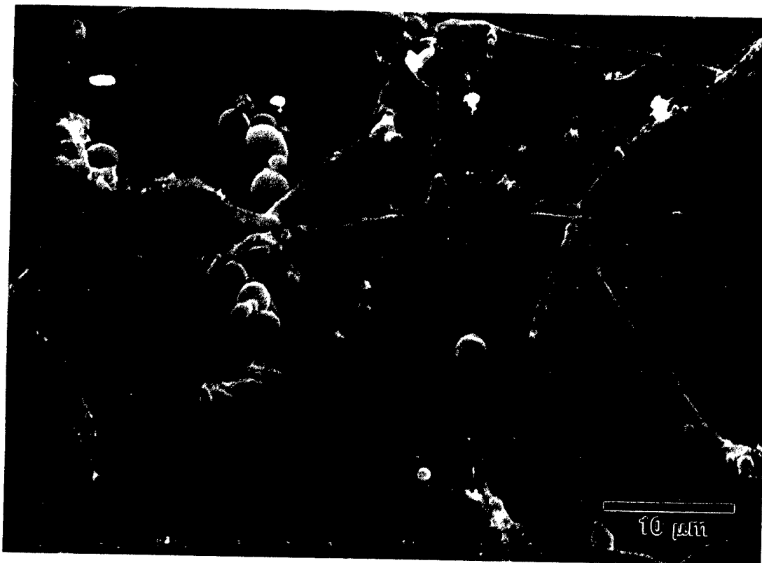
Figure 3. SEM micrograph of fungi on deteriorated polyimide films from an inoculated EIS cell after 7 days of inoculation
