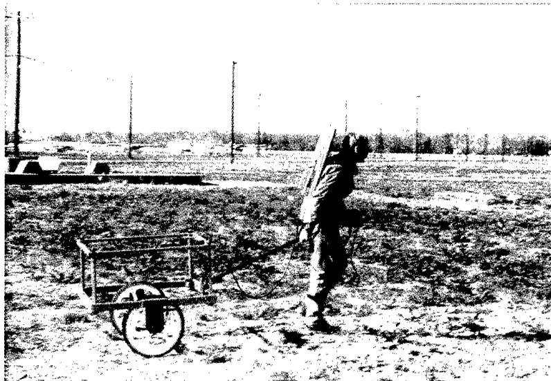
Figure 4. Geonics EM61 electromagnetic induction unit during a survey. The operator tows the antenna, while the backpack unit generates signals. Data are recorded on the hand-held datalogger.
